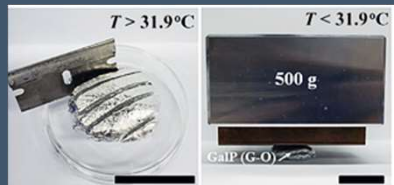
Figure 1: Gallium putty formed by mixing graphene oxide and gallium, forming a putty that easily can be cut at high temperatures but solid at low temperatures. (Wang et al., 2021)
