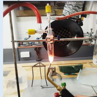
Figure 5: Gallium-gold mixture heated by propane-oxygen torch while under constant argon flow. Many thanks to Dr Robyn Hare for assisting us in making the glassware and use of the workshop for heating the sample.
